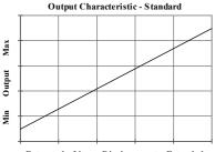
Retracted Linear Displacement Extended
